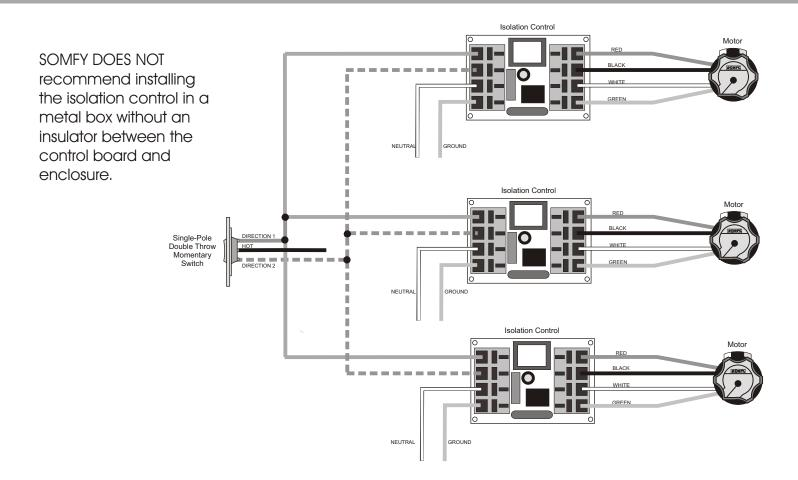
The Somfy Isolation Control can also be used whenever a single motor is operated by two or more switches. The control will keep the switches isolated and prevent both UP and DOWN directions from being activated simultaneously, thus protecting the motor. The control should only be used with Momentary Contact switches and 120V AC rated motors.
